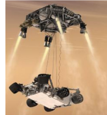
Sky crane hovers over the surface and lowers the Curiosity.
