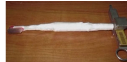
NASA photo of the toothbrush tool used to clean the metal shavings.
