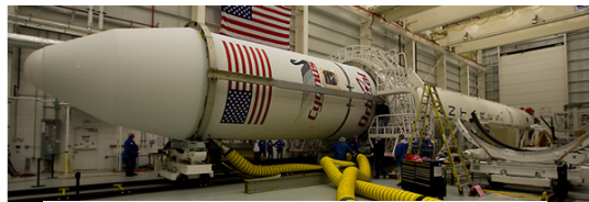
Installation of the rocket's payload fairing by Orbital Sciences Corp.'s Antares rocket on Oct. 23, 2014.
